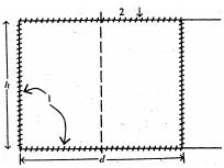
What is the value of the shape factor  $F_{12}$  in a cylindrical cavity of diameter d and height h between bottom face known as surface 1 and top flat surface known as surface 2?
