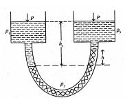
The balancing column shown in the above diagram contains 3 liquids of different densities  $\rho_1$ ,  $\rho_2$  and  $\rho_3$ . The liquid level of one Limb is h1 below the top level and
